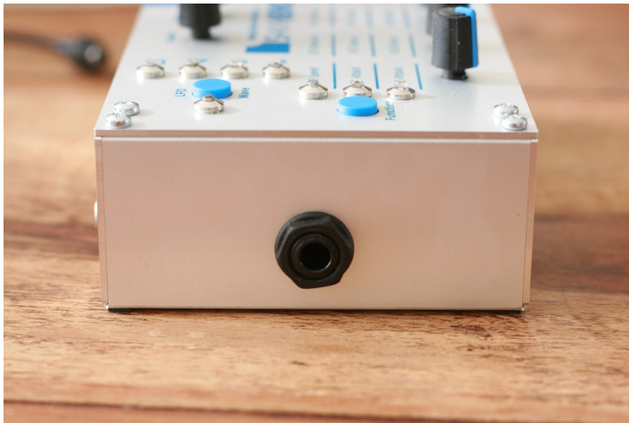
The left side of the Sawbench: the phono jack (audio out).
