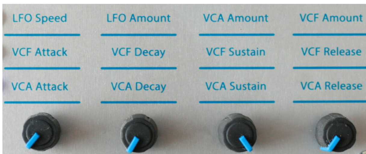
The ADSR knobs and their functions.
