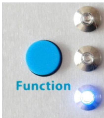
The function button and its three state LEDs.
