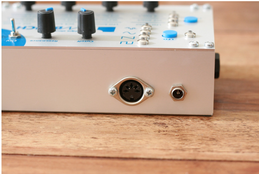
The back side of the Sawbench: MIDI in and power jacks.
